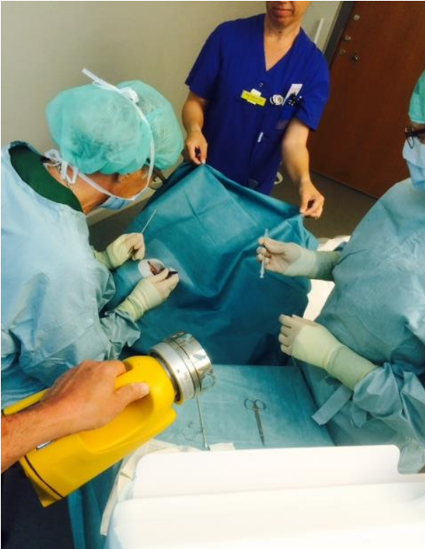
Simulated injection 12th of June CFU measurement of air cleanliness in the airflow from Operio between the instruments and injection site.
