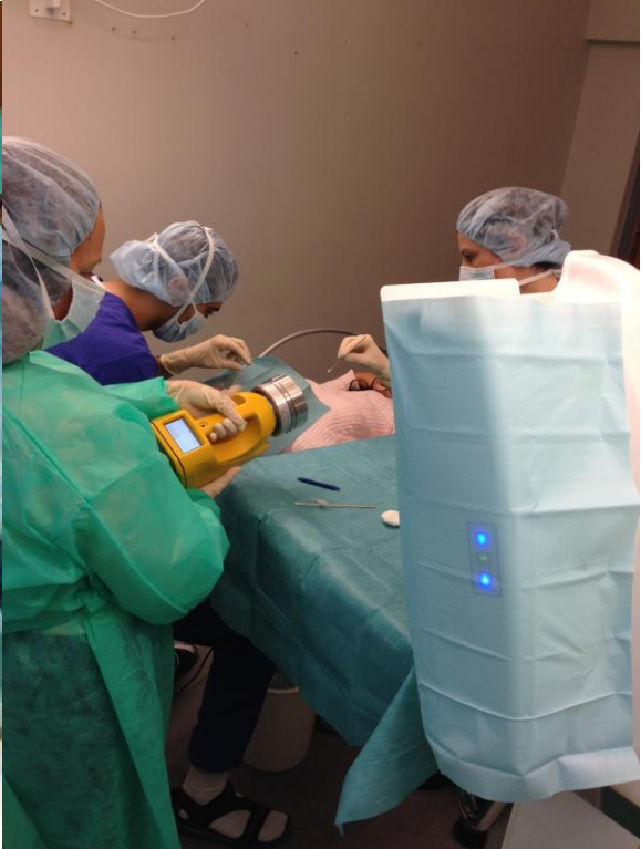
Authentic eye injection 6th of October CFU measurement of air cleanliness in the airflow from Operio between the instruments and injection site.
